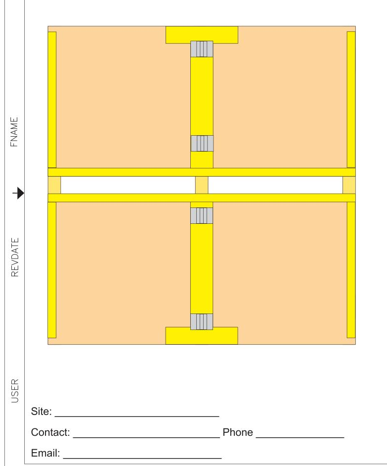
Per Pallet 2 - PT Fence Slat 1x6 3 - PT 2x4 x 46" 2 - Formboard Plywoo
